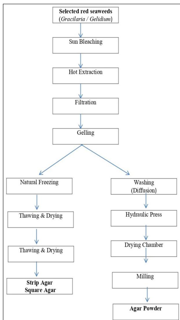
**Fig. 2:** Flow chart showing extraction of agar-agar from seaweeds (FAO, 1987)
