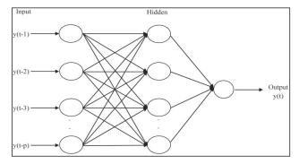
Fig. 1: Structure of Feed Forward Artificial Neural Network with single hidden layer
