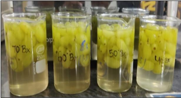
**Plate 4:** Grapes were dipped in the prepared solutions of 40°, 50°, 60° and 70° Bx
