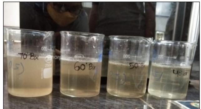
**Plate 3:** Prepared sugar solution of different concentrations of sugar
