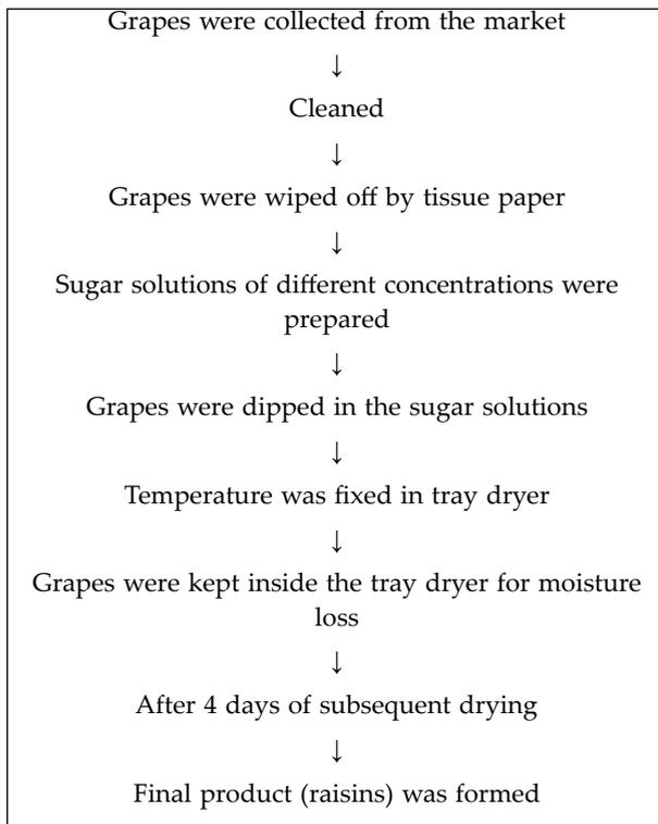
**Fig. 1:** Flow chart for processing of grapes to make raisins
