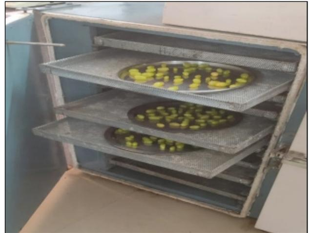
**Plate 5:** Grapes were kept inside the tray dryer for drying for 8h
